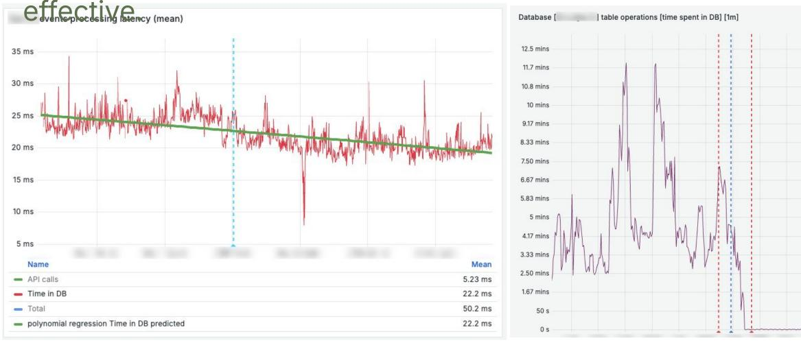
**Solution:** We had to rewrite number of queries to use application-level cache. In resulted in ~4ms (15%) latency improvement.
