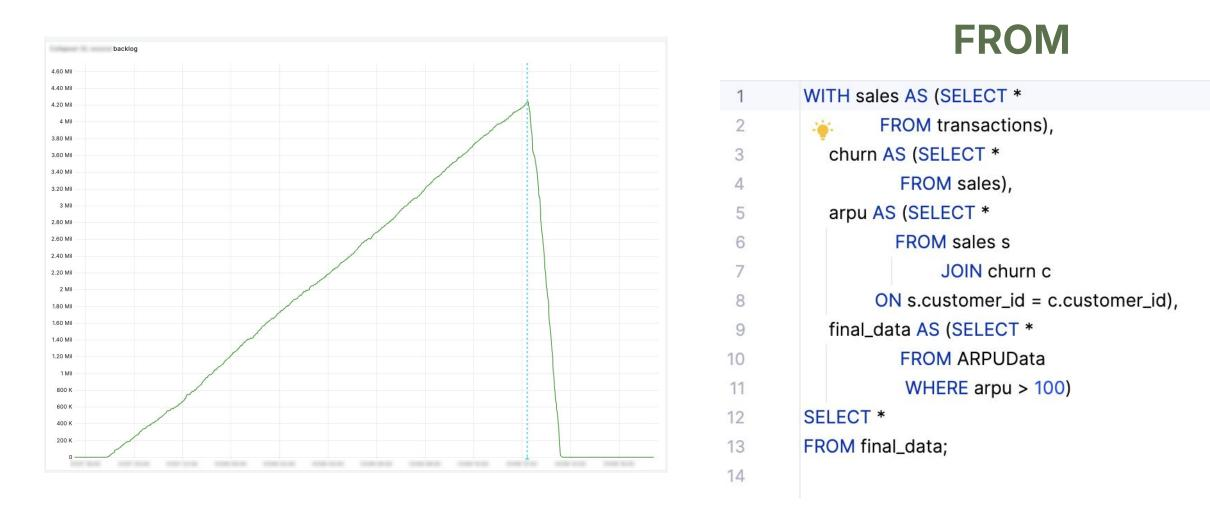
Solution: We broke down complex, 5-queries CTE into smaller queries to help database in choosing a right query plan. P.S. Avoid batch processes!
