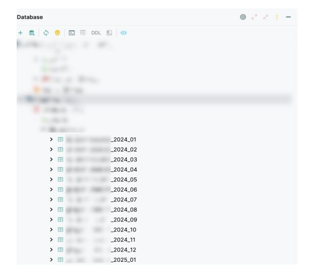
**Solution:** We partitioned large tables by **monthly chunks**, easing job for database management tasks and optimise data access. Duration of **maintenance tasks reduced more than 10 times.**
